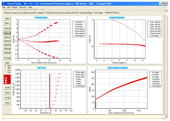
Figure 6-1 Typical Output using Visual Plumes Model
