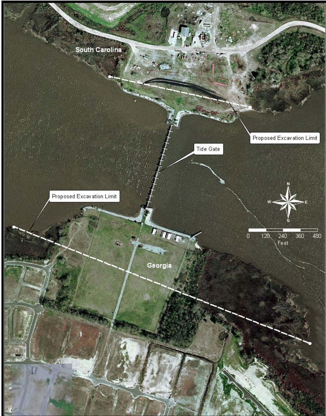
Figure 3-3. Proposed excavation areas near the Tidegate.
