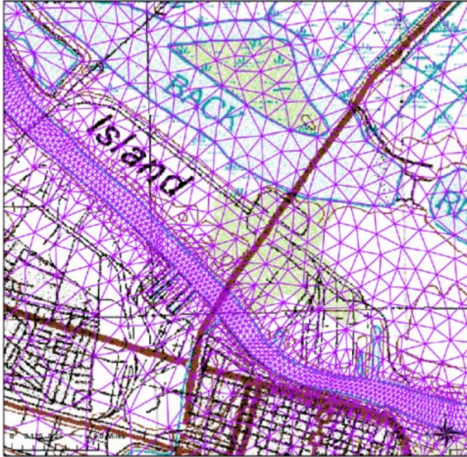
Figure 4-7. Detailed view of finite element grid in the Savannah area.
