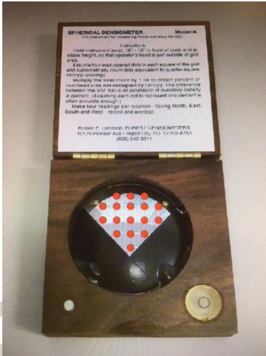
Figure 2. Locations on the face of the densiometer used to assess stream channel shading (vis a vis canopy coverage).
