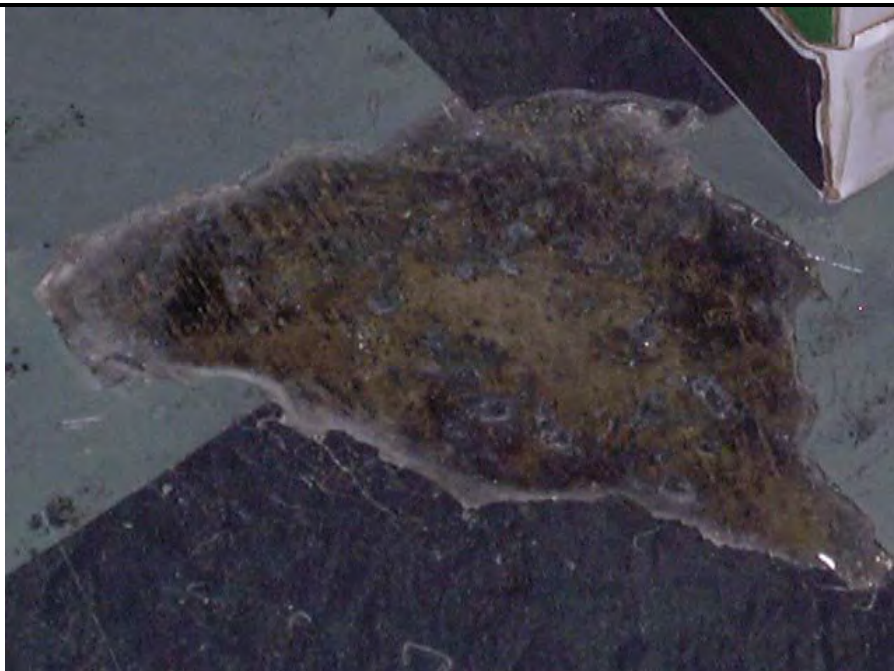
Photo 20: 12" x 12" black vinyl floor tile/ mastic– AFRC Building Room 120 (2 Layers of Tile is positive for Asbestos, 2 Layers of Mastic is positive for Asbestos)
