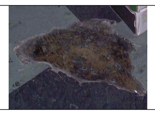
Photo 20: 12" x 12" black vinyl floor tile/ mastic (2 Layers of Tile is positive for Asbestos, 2 Layers of Mastic is positive for Asbestos)
