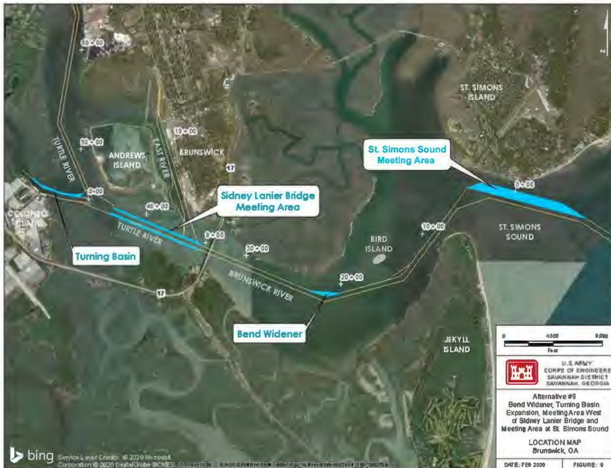
Figure 26. Alternative 9 – Bend widener, turning basin expansion, meeting area west of the Sidney Lanier Bridge, and meeting area at St. Simons Sound
