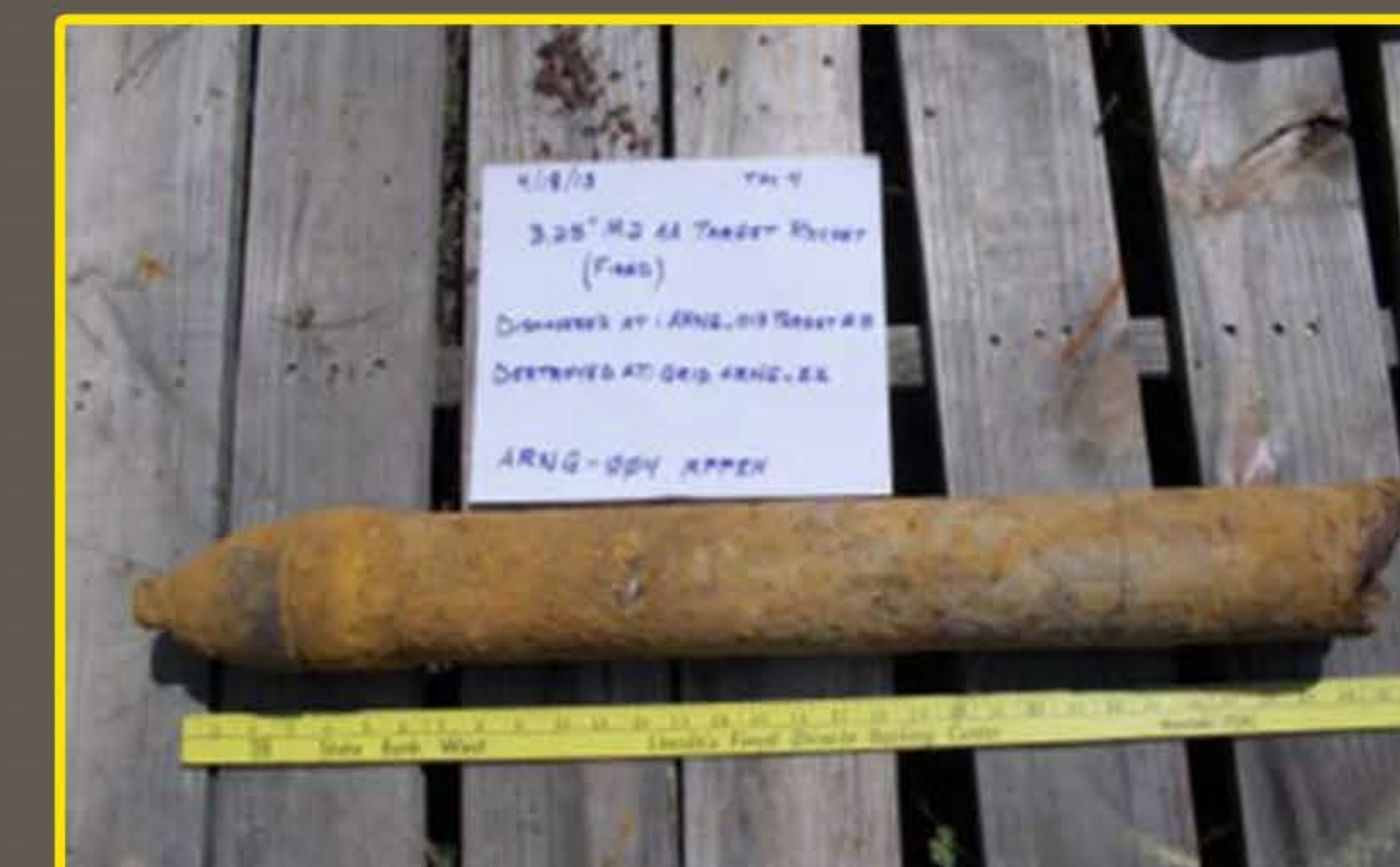
M2 3.25" Anti-Aircraft Rocket
