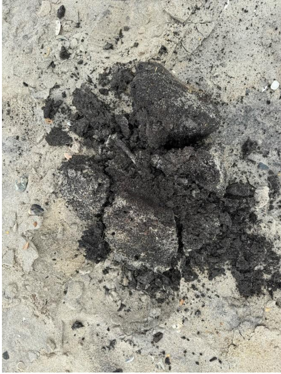
Photo 16 - Example of larger chunk of "peat-like" material found on beach near southern leach field. Material was light, friable, had visible organic material and organic odor.
