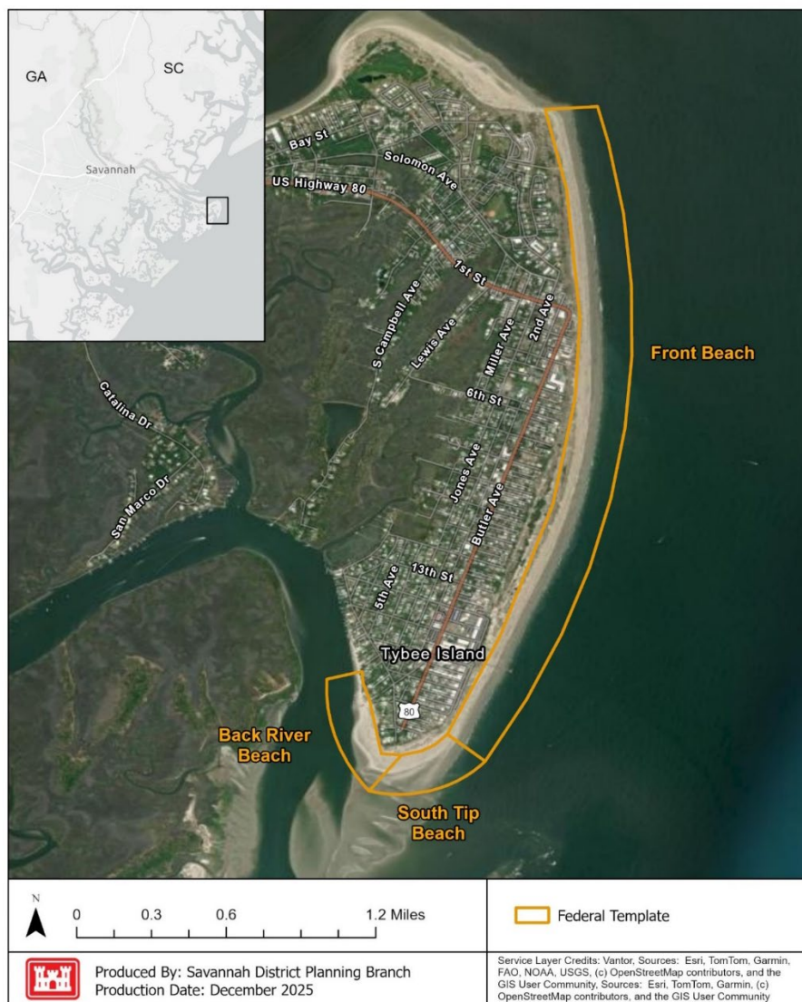
Figure 1. TISPP approximate Federal template for beach renourishment.
