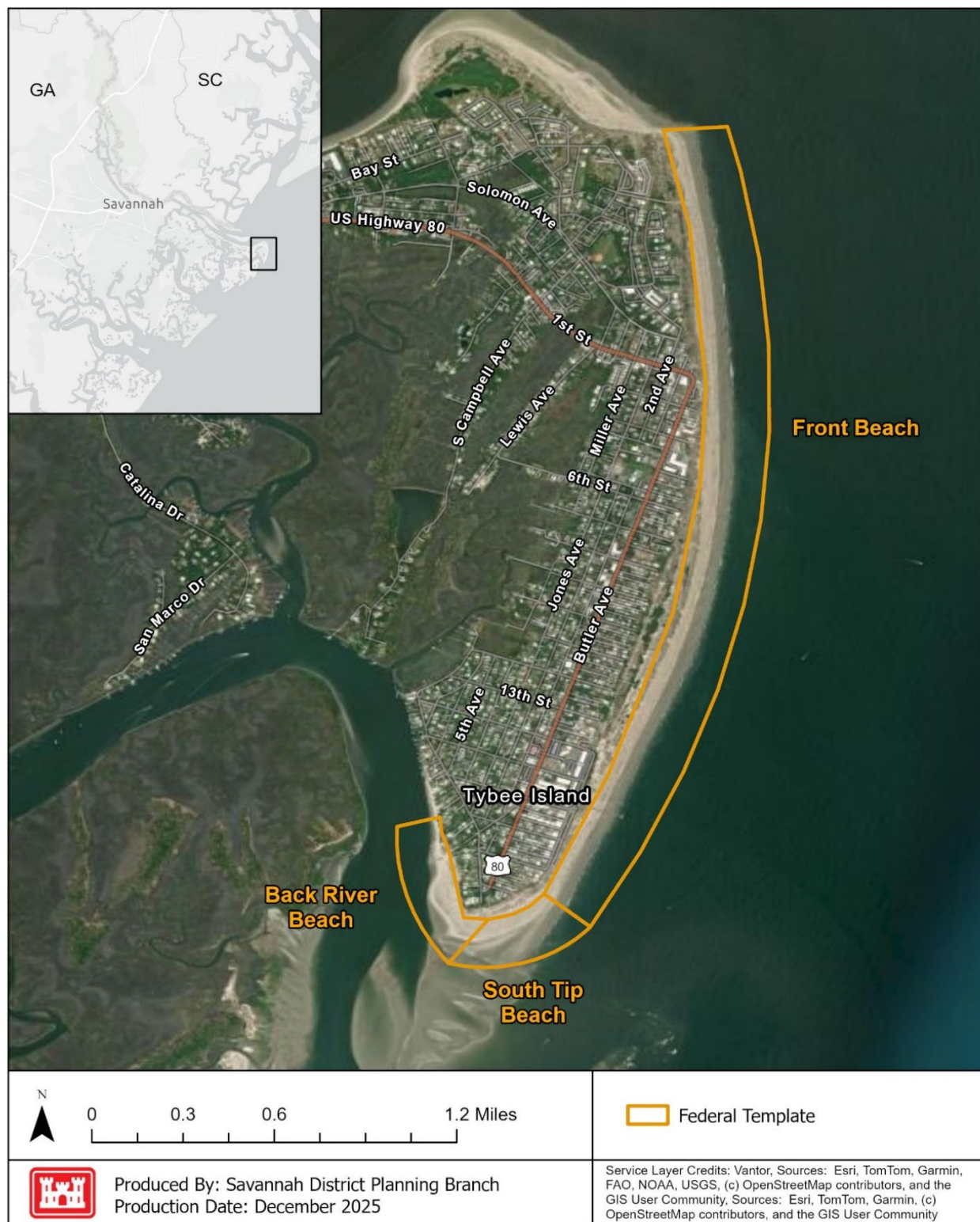
Figure 1. TISPP approximate Federal template for beach renourishment.
