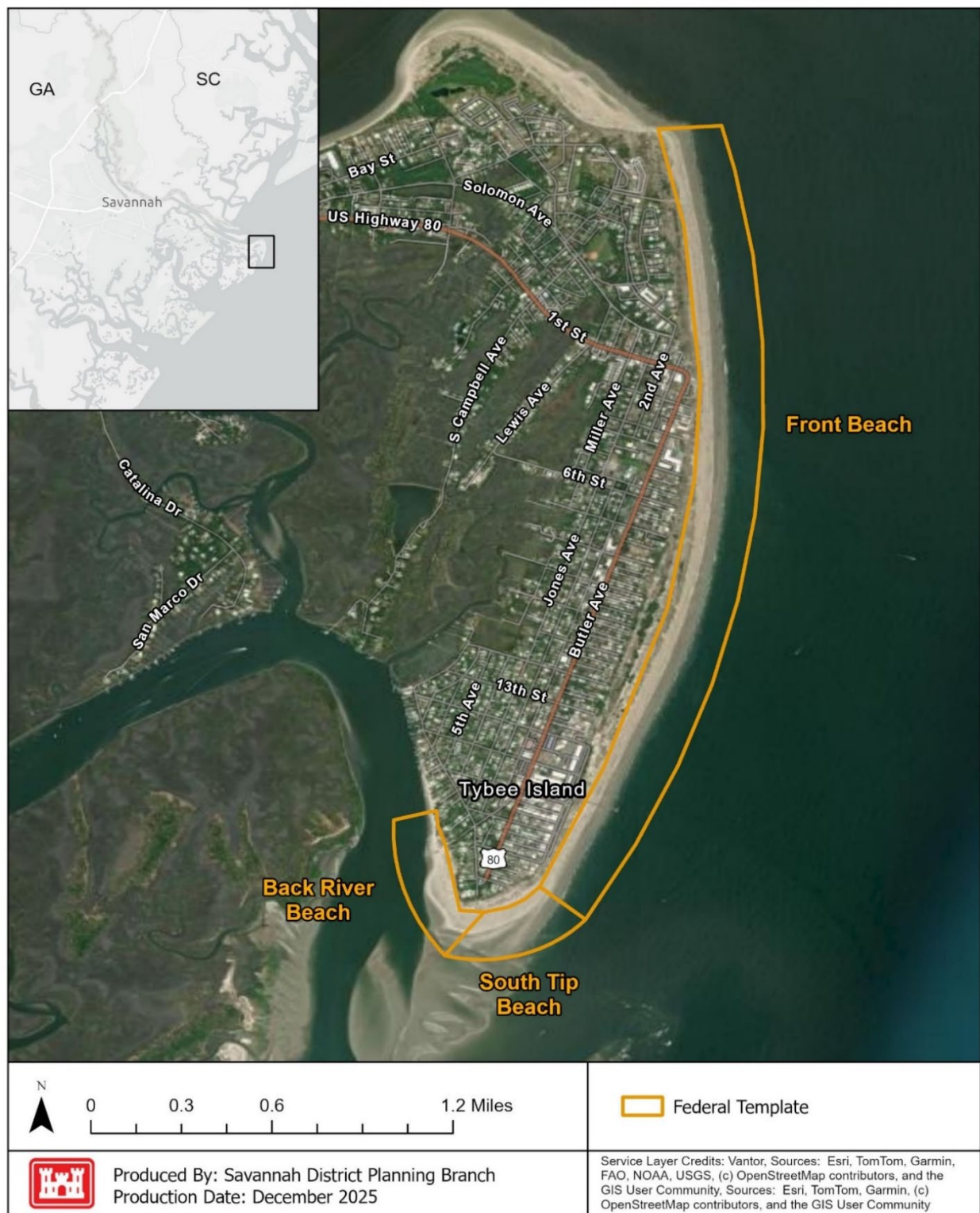
Figure 1. TISPP approximate Federal template for beach renourishment.
