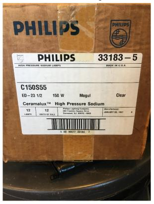
Photo 17: Case of bulbs labeled High Pressure Sodium
