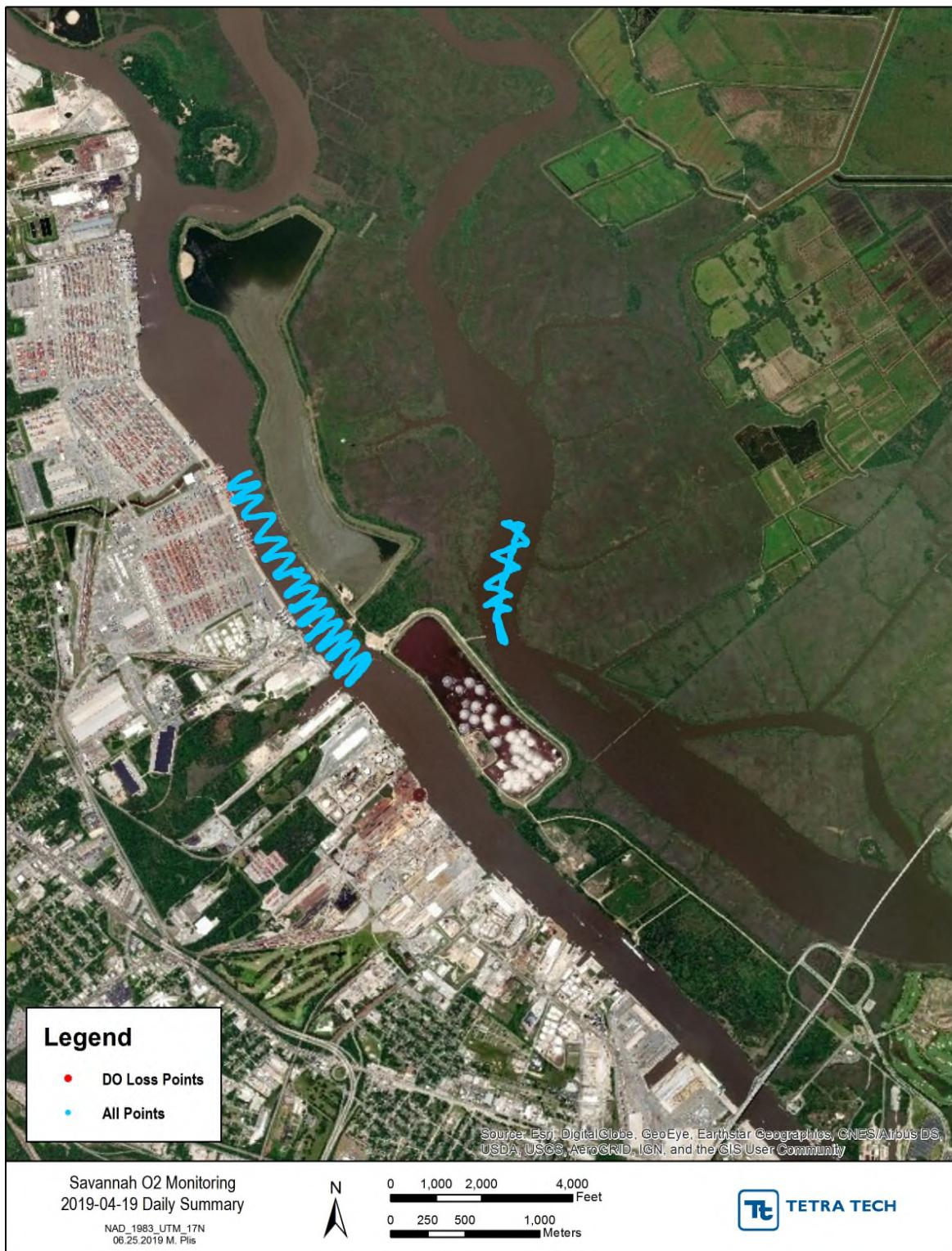
**Figure H-73** April 19, 2019 Intermittent Surface data (blue) and Intermittent DO Loss data (red) for lower Front River and Back River
