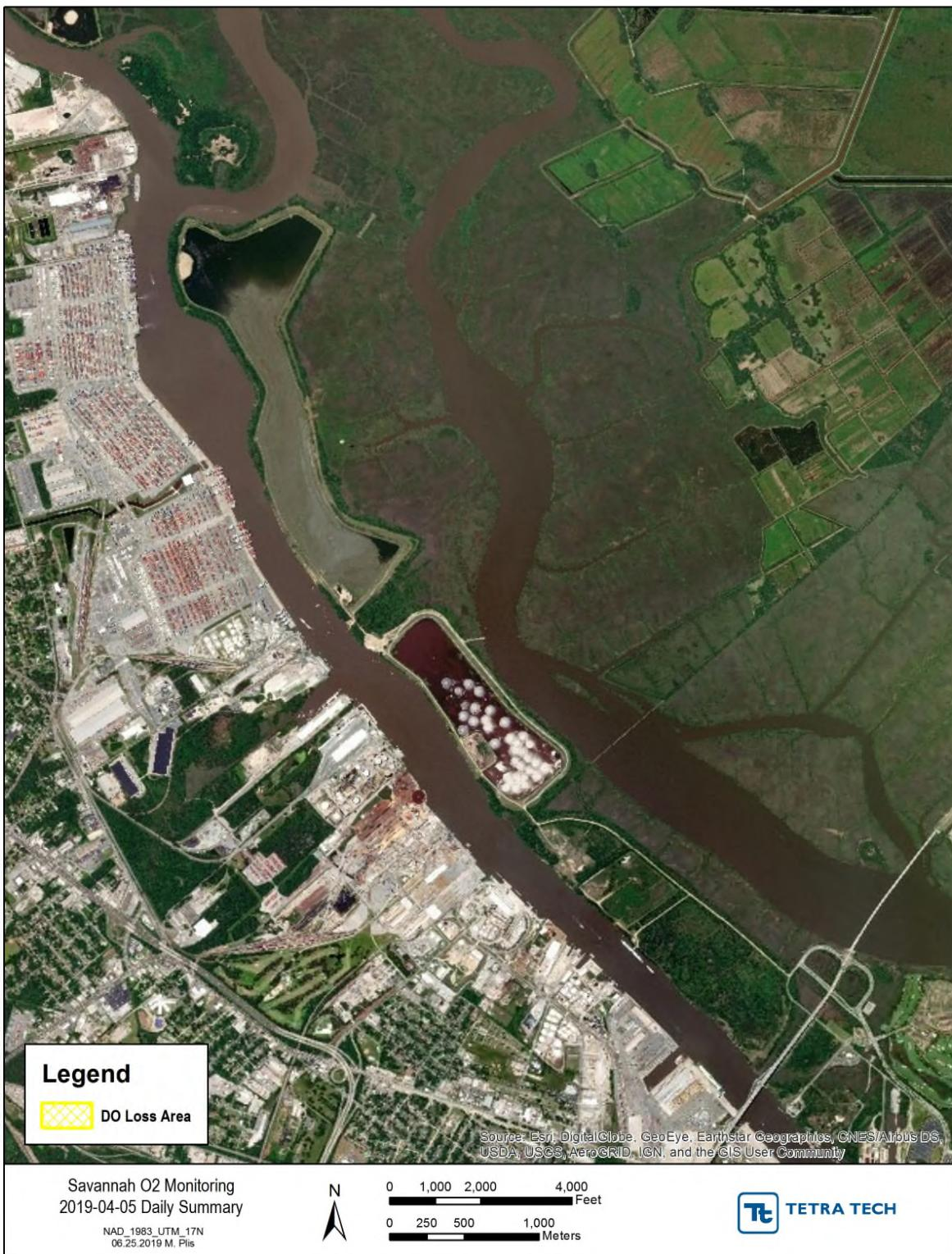
**Figure H-46** April 5, 2019 Daily Intermittent data DO Loss Area for lower Front River and Back River
