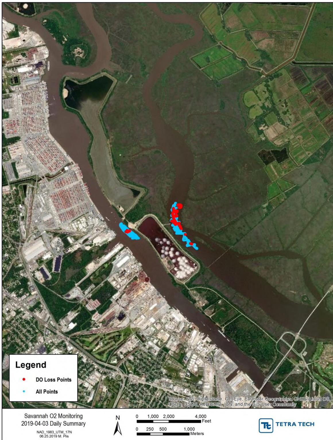
**Figure H-41** April 3, 2019 Intermittent Surface data (blue) and Intermittent DO Loss data (red) for lower Front River and Back River
