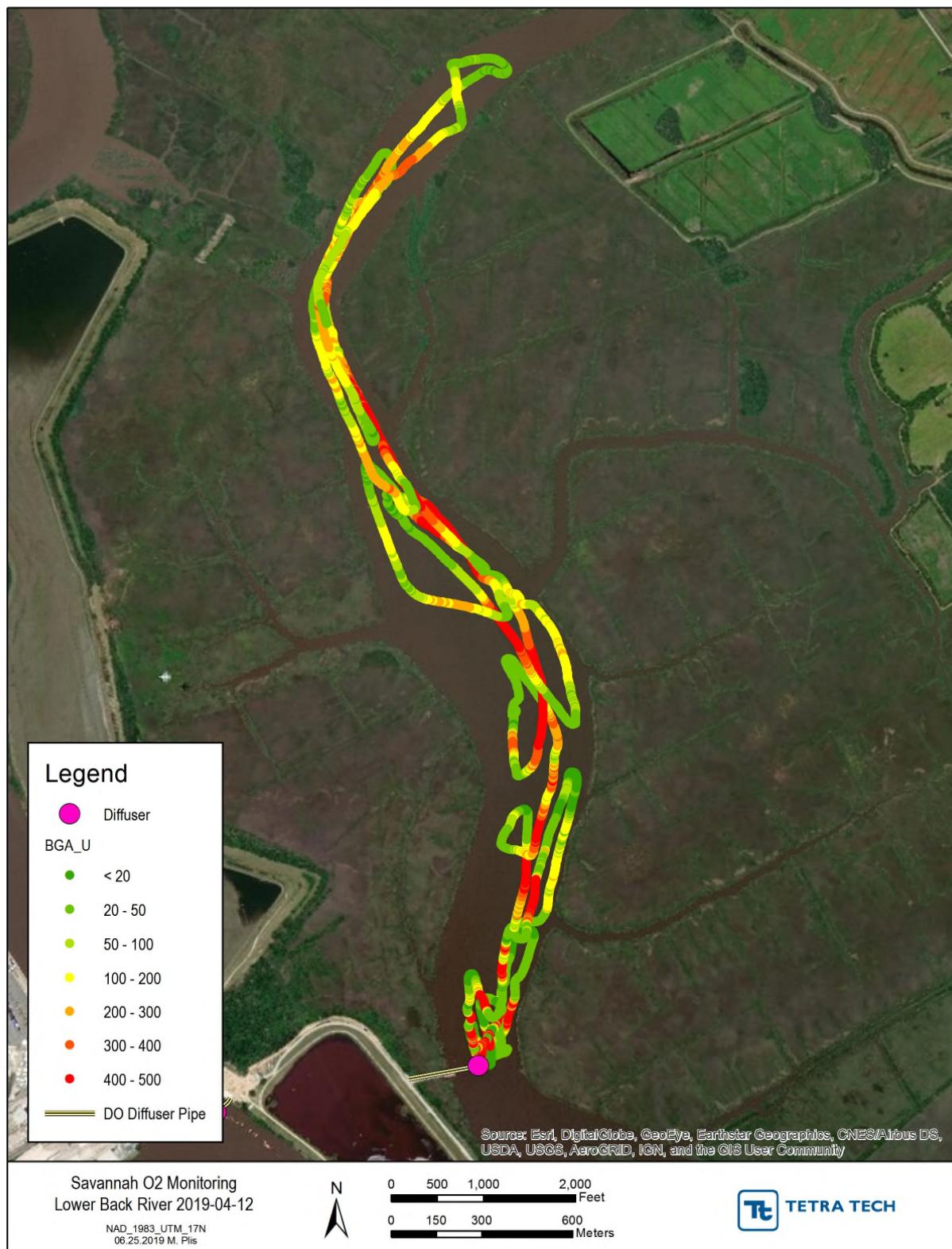
**Figure G-5** Back River April 12, 2019 ebb tide dye drift boat 2 points
