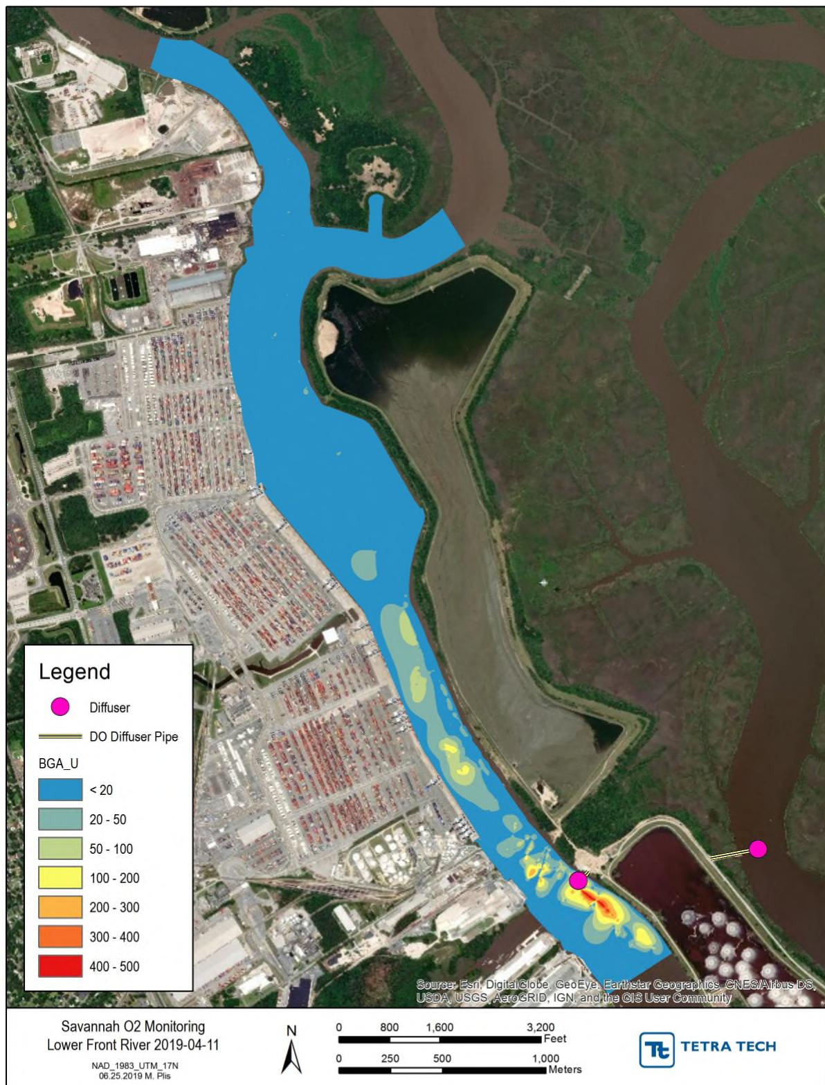
**Figure G-22** Front River April 11, 2019 ebb tide dye drift boat 2 raster interpolation
