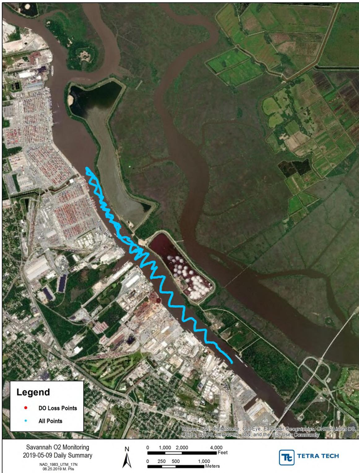
**Figure H-113** May 9, 2019 Intermittent Surface data (blue) and Intermittent DO Loss data (red) for lower Front River and Back River
