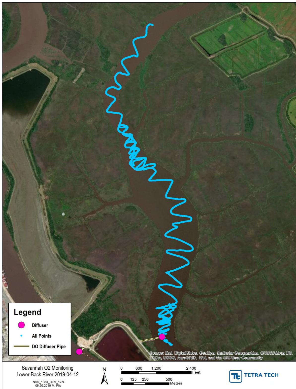
**Figure D-27** Back River April 12, 2019 ebb tide dye drift location map boat 1
