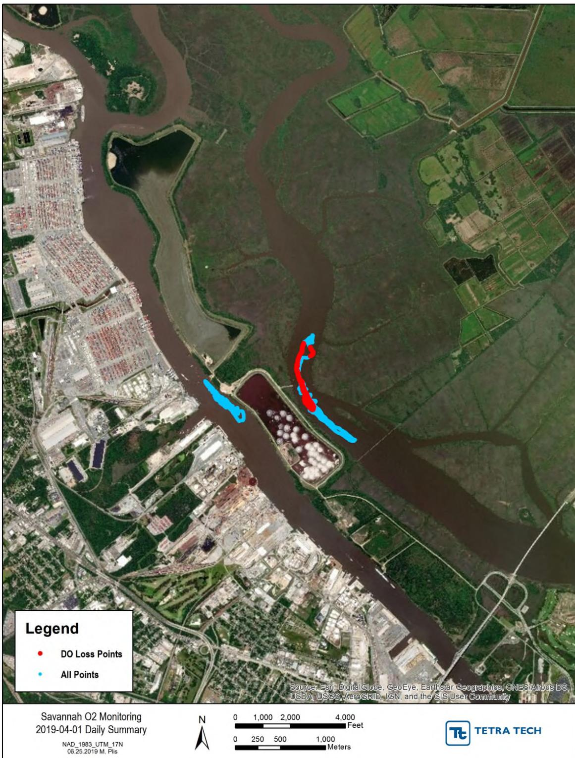
**Figure H-37** April 1, 2019 Intermittent Surface data (blue) and Intermittent DO Loss data (red) for lower Front River and Back River
