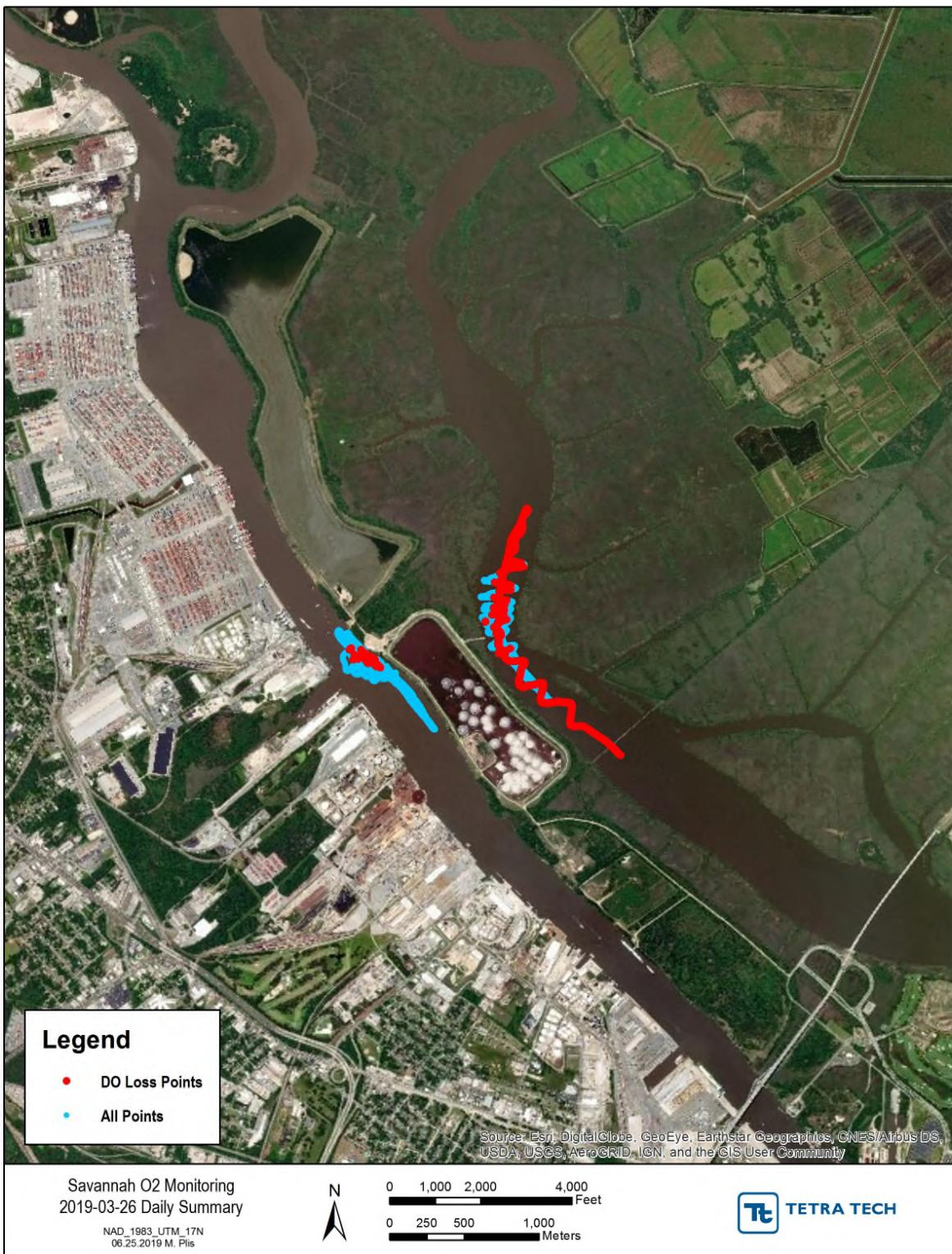
**Figure H-25** March 26, 2019 Intermittent Surface data (blue) and Intermittent DO Loss data (red) for lower Front River and Back River
