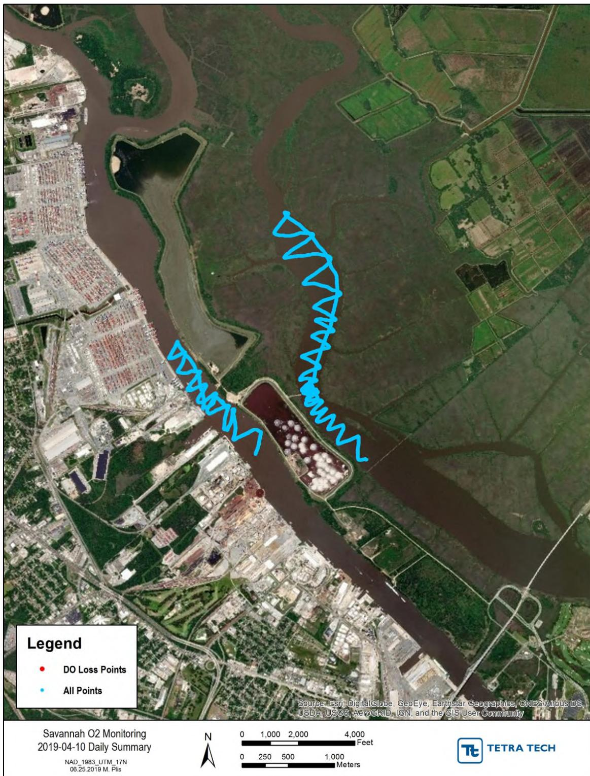
**Figure H-55** April 10, 2019 Intermittent Surface data (blue) and Intermittent DO Loss data (red) for lower Front River and Back River
