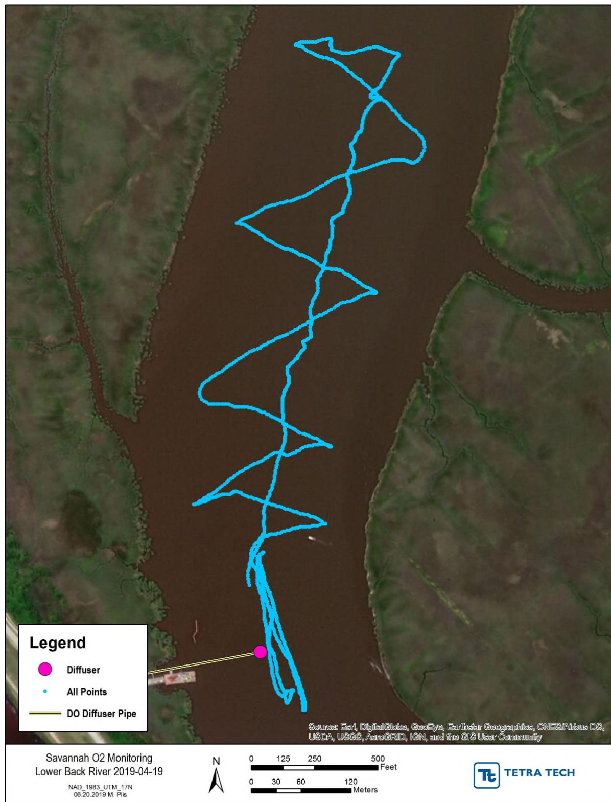
**Figure D-35** Back River April 19, 2019 flood tide drift location map
