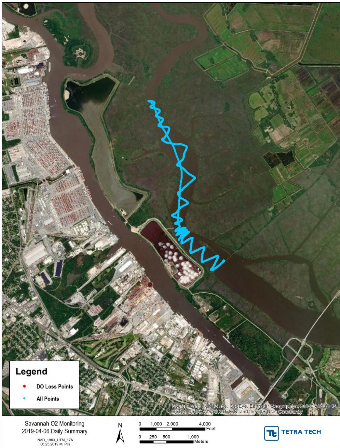
**Figure H-47** April 6, 2019 Intermittent Surface data (blue) and Intermittent DO Loss data (red) for lower Front River and Back River
