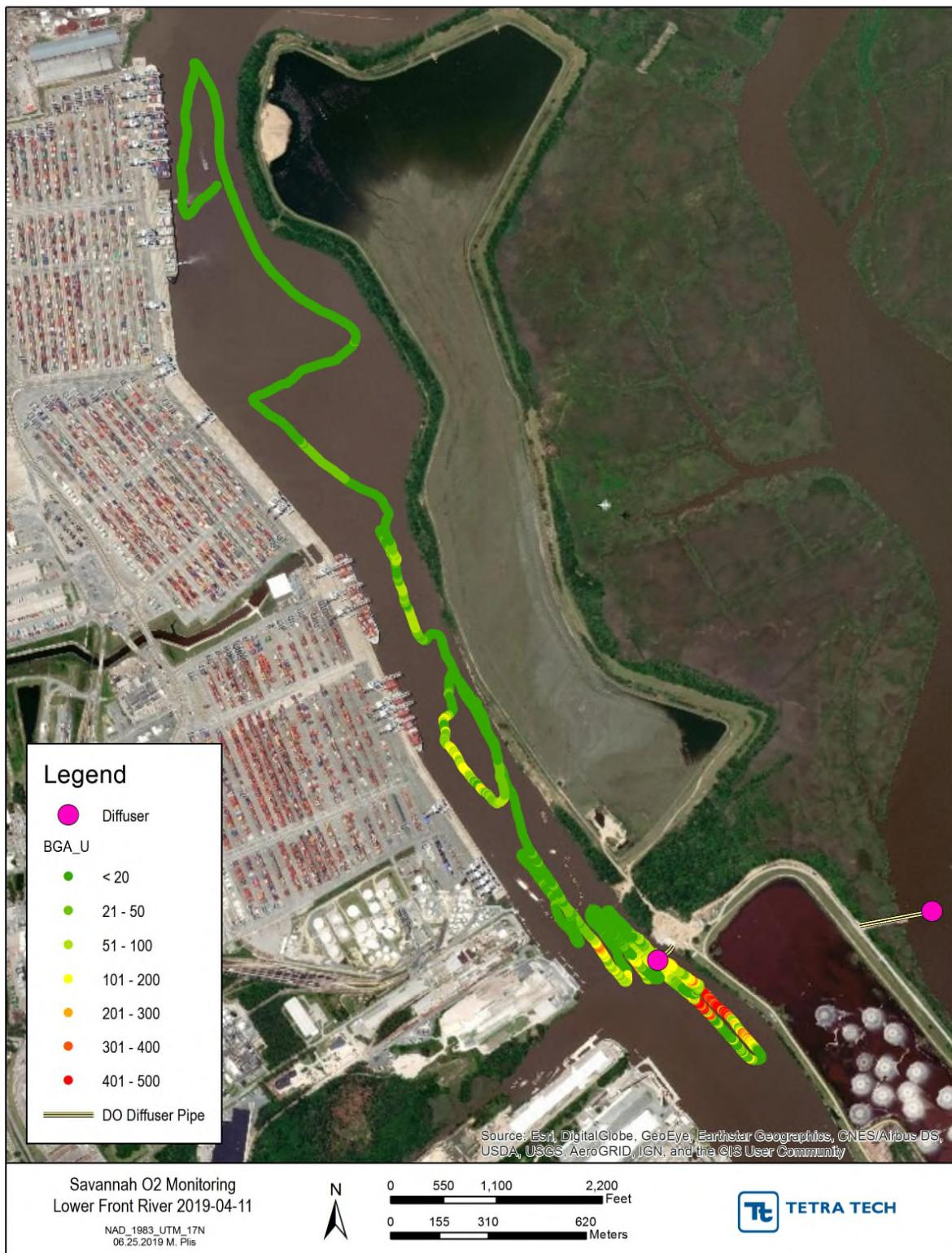
**Figure G-17** Front River April 11, 2019 ebb tide dye drift boat 1 period 1 points
