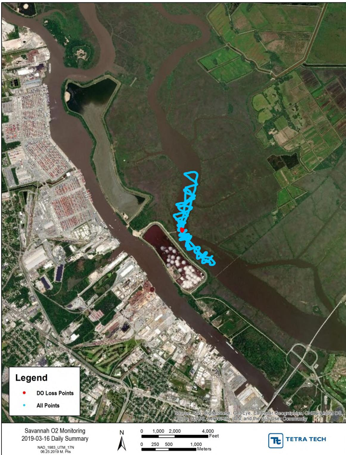
**Figure H-5** March 16, 2019 Intermittent Surface data (blue) and Intermittent DO Loss data (red) for lower Front River and Back River
