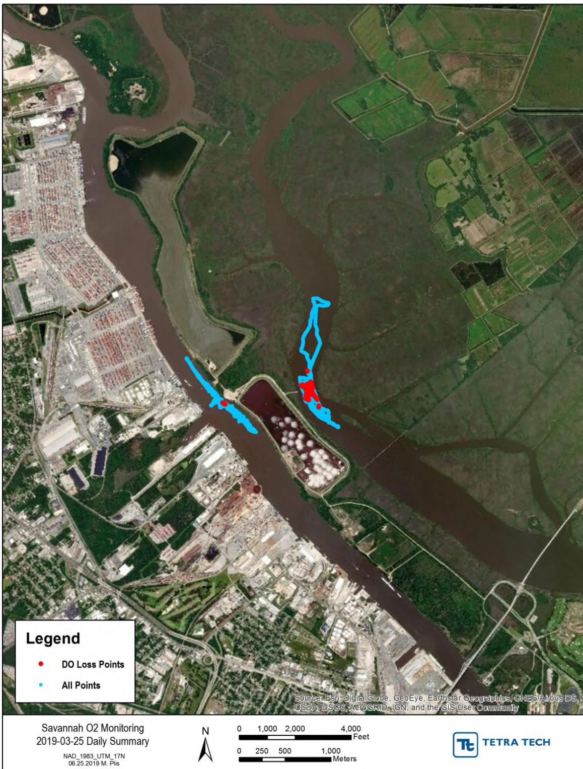
**Figure H-23** March 25, 2019 Intermittent Surface data (blue) and Intermittent DO Loss data (red) for lower Front River and Back River
