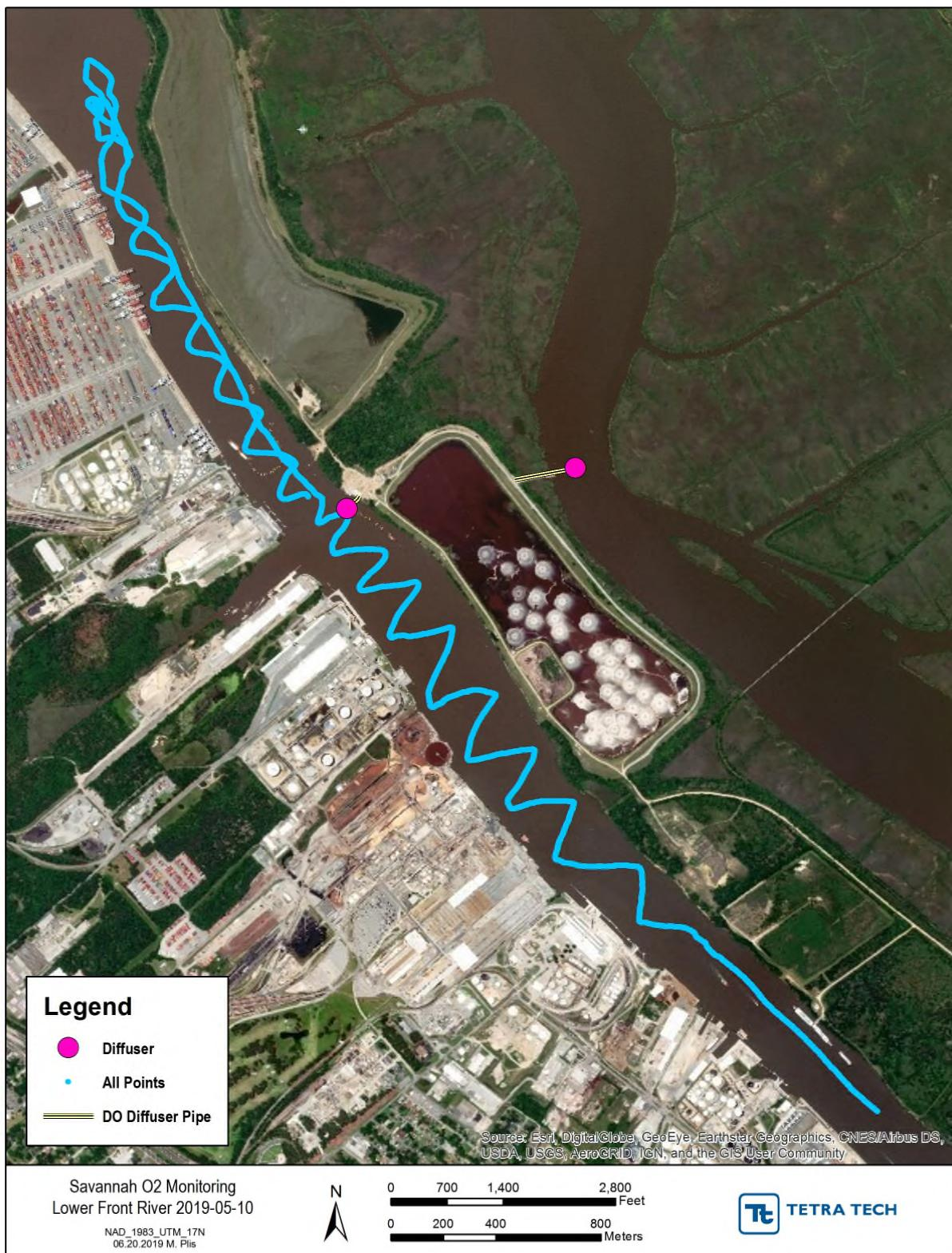
**Figure D-125** Front River May 10, 2019 flood tide drift location map
