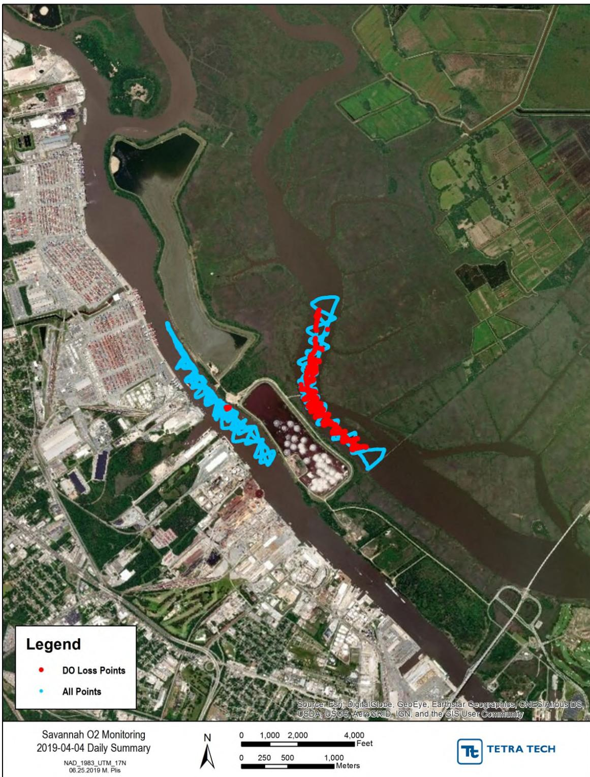
**Figure H-43** April 4, 2019 Intermittent Surface data (blue) and Intermittent DO Loss data (red) for lower Front River and Back River
