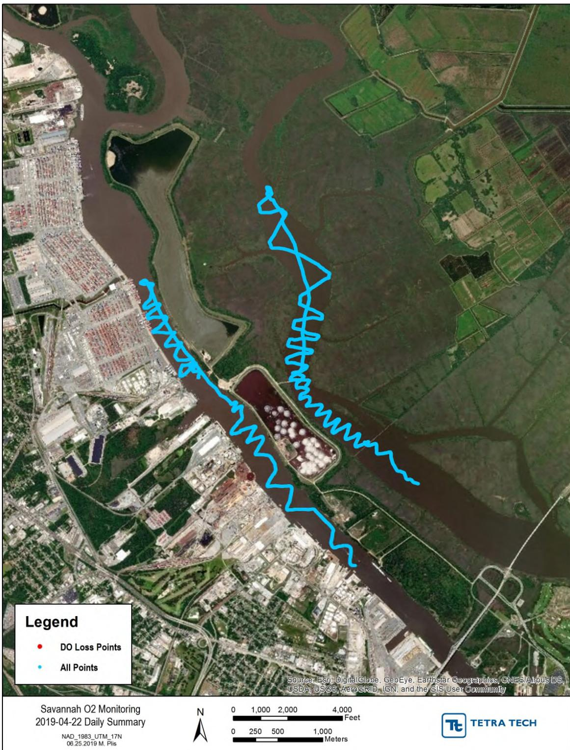
**Figure H-79** April 22, 2019 Intermittent Surface data (blue) and Intermittent DO Loss data (red) for lower Front River and Back River
