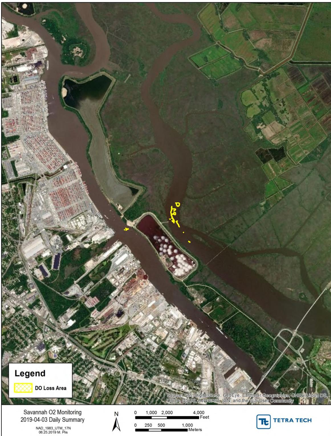
**Figure H-42** April 3, 2019 Daily Intermittent data DO Loss Area for lower Front River and Back River
