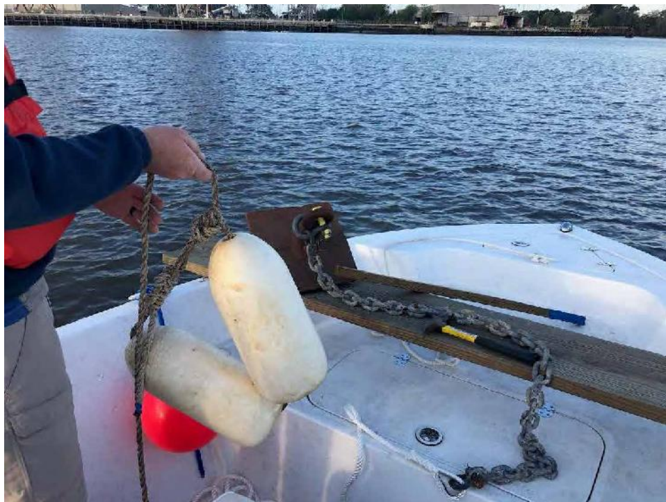
Photo 2 – Buoy and Dormor configuration
