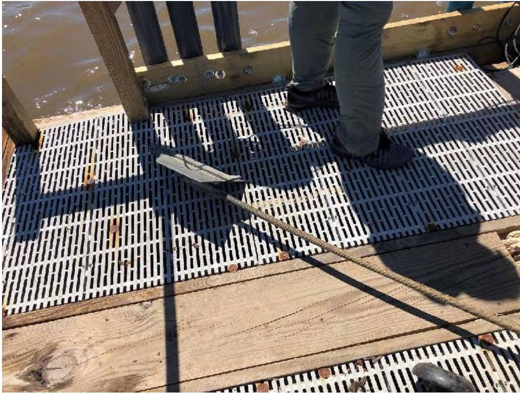
Photo 5 – Southeast Manta ray anchor extracted from river.
