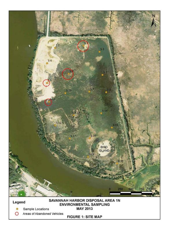
Fifty-four samples were collected from the 19 sampling locations on May 14 and 15, 2013. Samples were taken from the ground surface (elevations varying between 22 and 13 feet Mean Lower Low Water (MLLW)) down to a bottom elevation of either 10 or 6 feet MLLW, depending on location The water table at DMCA 1N is approximately 6 feet MLLW. In most cases, samples were composited every 4 feet until reaching the bottom depth (table 1).
