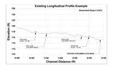
(iii) Longitudinal profile diagram of the proposed culvert, including the proposed culvert slope, type and size, invert elevations, and embedded depth; elevation of the existing streambed (along the thalweg); and locations of channel excavation (i.e., constructed channel between the existing stream channel and proposed culvert), headwalls, outlet protection, and energy dissipaters, as applicable.
