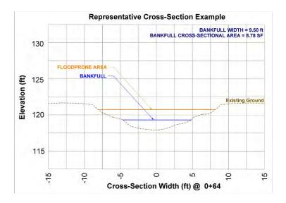
(v) Cross-sectional diagrams of the proposed culvert inlet and outlet, including location of the culvert in the stream channel; culvert type and size; proposed road surface and areas of cut and fill; elevations of the culvert invert and stream bottom and stream channel bed and banks, bankfull, and floodprone area (i.e., 2x the maximum bankfull depth). The diagram shall note the proposed bankfull cross-sectional area. The X and Y axis must be at the same scale.
