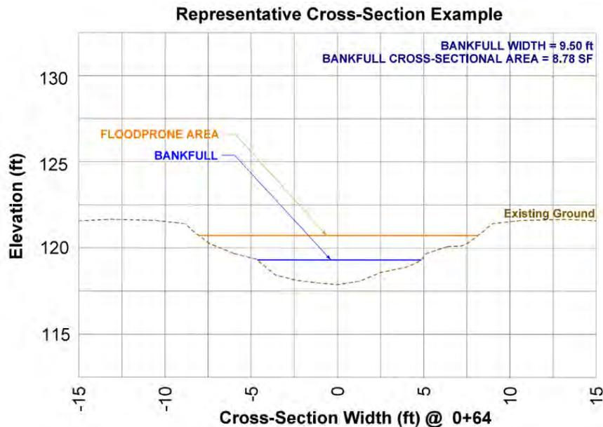
(v) Cross-sectional diagrams of the proposed culvert inlet and outlet, including location of the culvert in the stream channel; culvert type and size; proposed road surface and areas of cut and fill; and elevations of the culvert invert and stream bottom and stream channel bed and banks, bankfull, and floodprone area (i.e., 2x the maximum bankfull depth). The diagram shall note the proposed bankfull cross-sectional area. The X and Y axis must be at the same scale.
