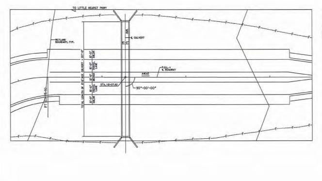
PROPOSED BRIDGE CONSISTS OF 1 - 137'-0" 8'X8' CONCRETE BOX CULVERT - GA. 5TD. 2401
