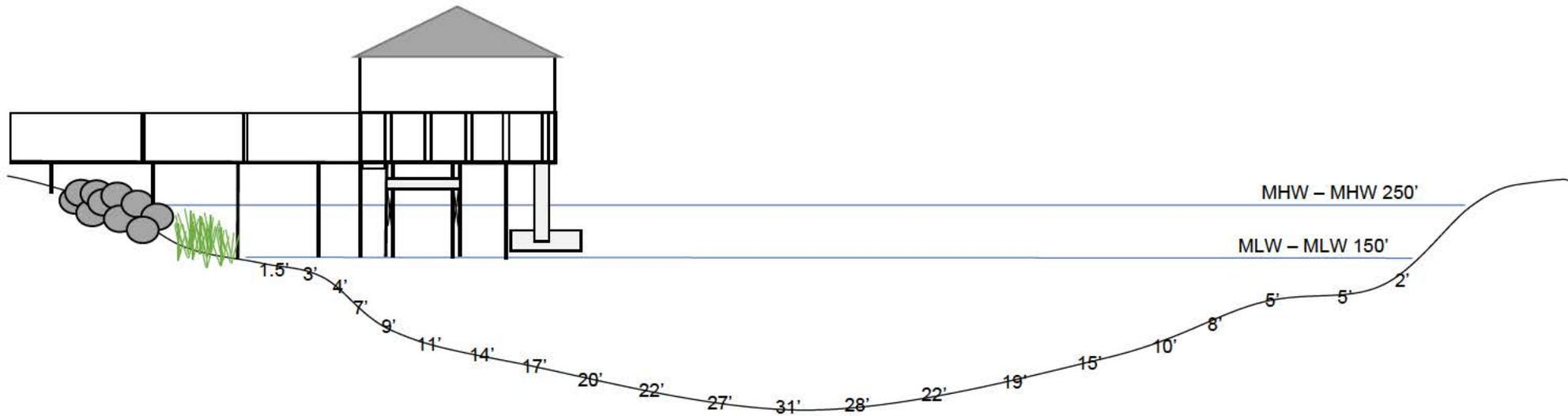
Note: The measurements should be taken at a standard number of feet across the entirety of the waterbody at MLW. (i.e. every 5 ft.)
