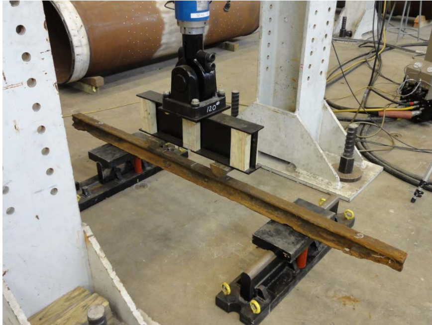
Figure 10: Test setup for rail flexural test.
