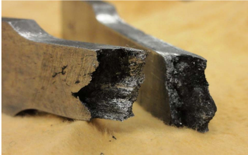
Figure 9: Failure location view of axial tensile specimen (4-1).
