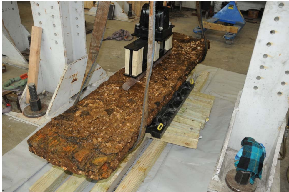
Figure 1: View of rail casement split test setup.
