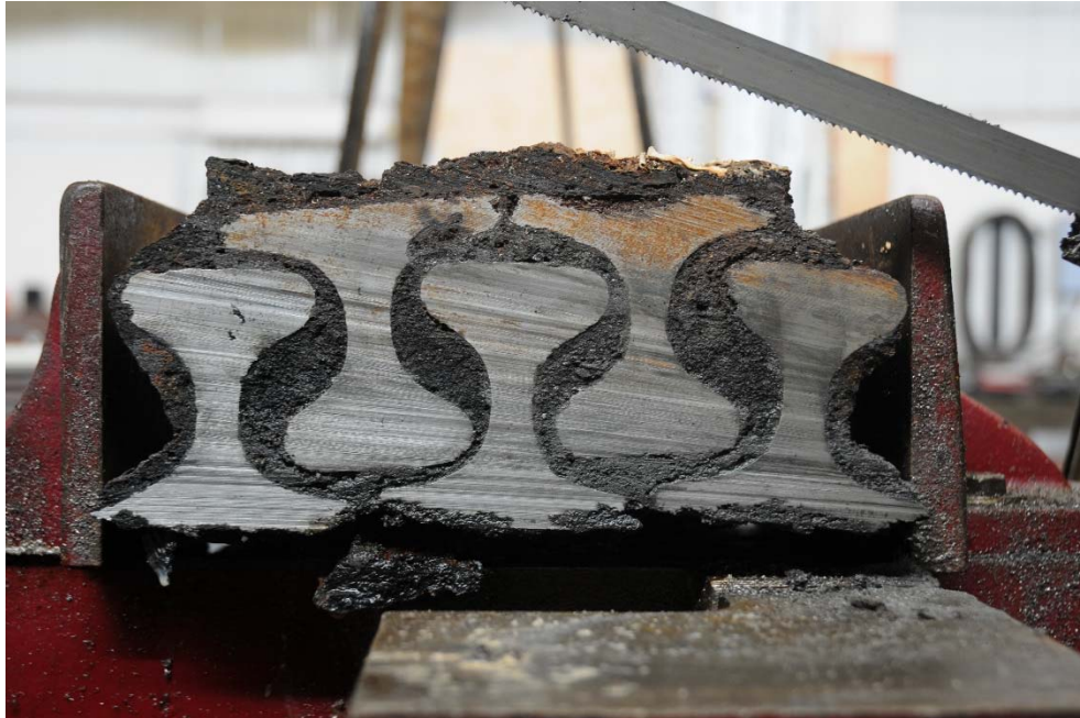
Figure 2: Cross-sectional view of five rails after cutting.
