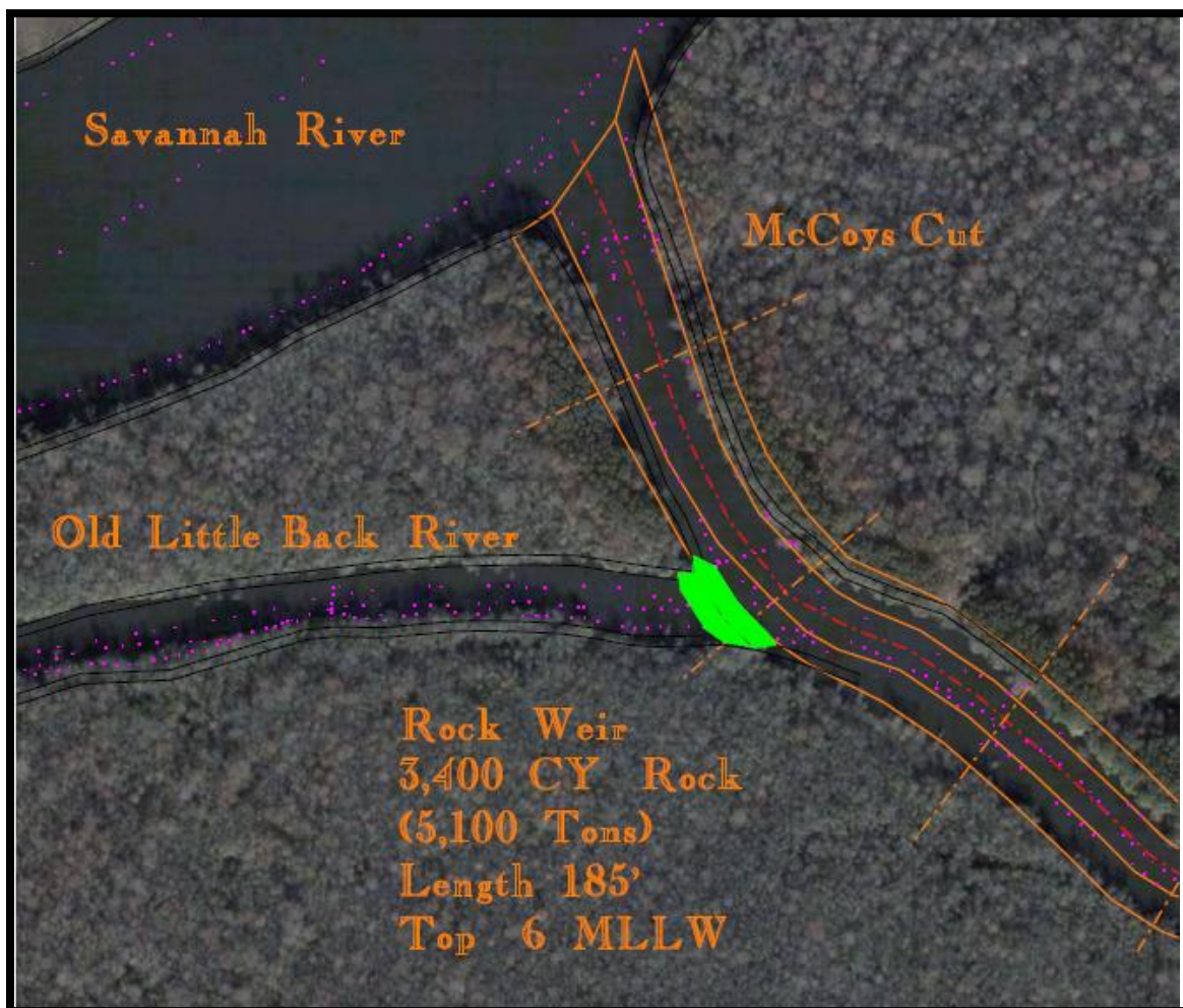
Figure 37. Plug in Old Little Back River (western arm of McCoys Cut).
