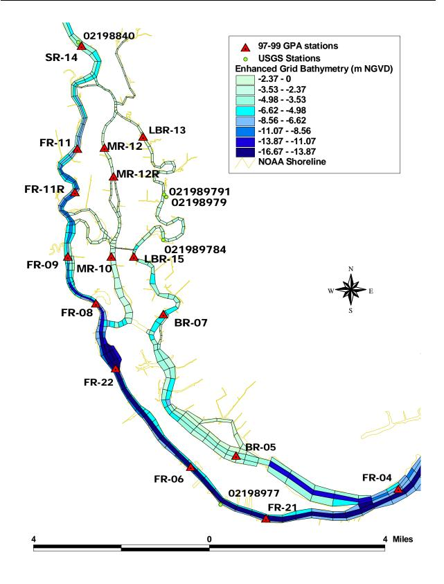
Figure 2-2 Model Grid and Bathymetry in the Upper Estuary
