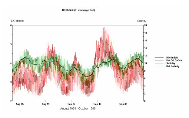
Figure 9 – DO deficit versus salinity at IP discharge (MA = Moving Average)
