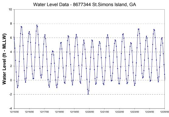
Figure 14 – Water level data measured at St Simons Island NOAA gage
