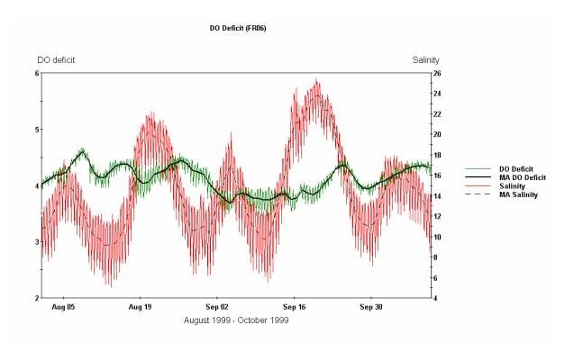
Figure 11 – DO deficit versus salinity at FR-06, downstream of IP discharge near Talmadge Bridge (MA = Moving Average)
