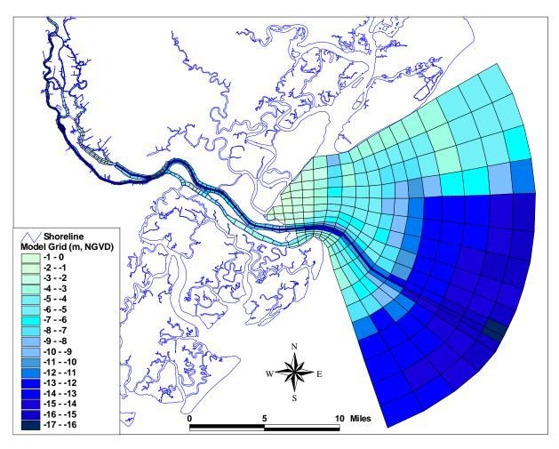
Figure 2-1 Model Grid and Bathymetry
