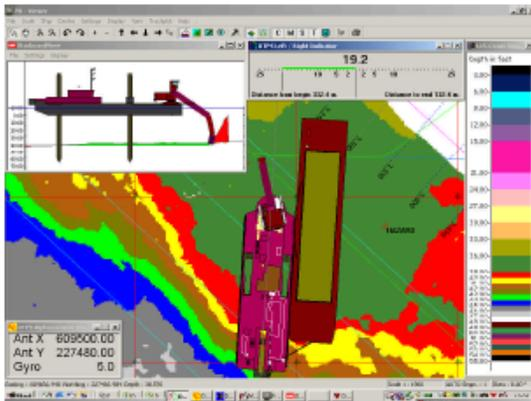
The DTPS system shows on-line the excavator in the Digital Terrain Model (DTM) with contours. The DTM or Bathymetric view with geographical co-ordinates can be rotated on-line by the operator and is also capable to store default views. The alphanumeric window shows all relevant data. The DTPS systems communicate bi-directional with the XPM. All XPM sensor data is converted to absolute position data and transferred back to the XPM.
