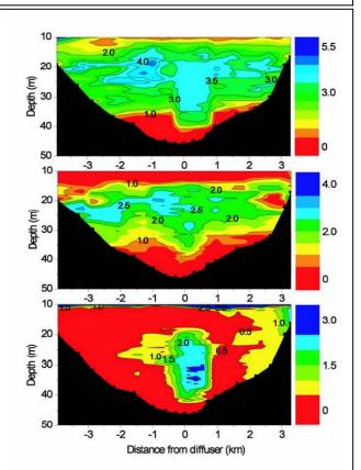
**Figure 8.** The (top) 24 July, (middle) 16 August, and (bottom) 27 September 2001 DO contours (g m<sup>-3</sup>). Note different scales. The *x* axis zero point is located at the center of the 300-m-diameter diffuser ring. The contours were interpolated from 18 CTD profiles (locations indicated by black squares at the bottom of the plots) sampled along the centerline of the lake (see Figure 2 map showing 18 sampling stations).
