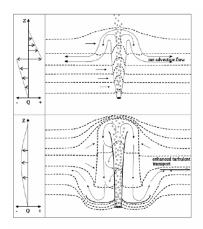
Figure 11. (top) Traditional plume model approach and (bottom) new model concept of plume behavior and shortcircuiting in deep lakes (not to scale). Dashed line indicates constant temperature isopleths demonstrating near-field alteration. Left axis shows approximate far-field vertical compensation flow rate distribution (see Figure 12).
