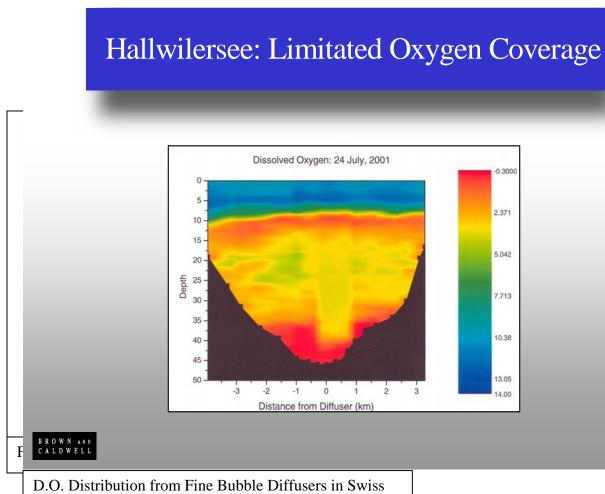
Lake – Note no D.O. at sediment interface below diffuser
