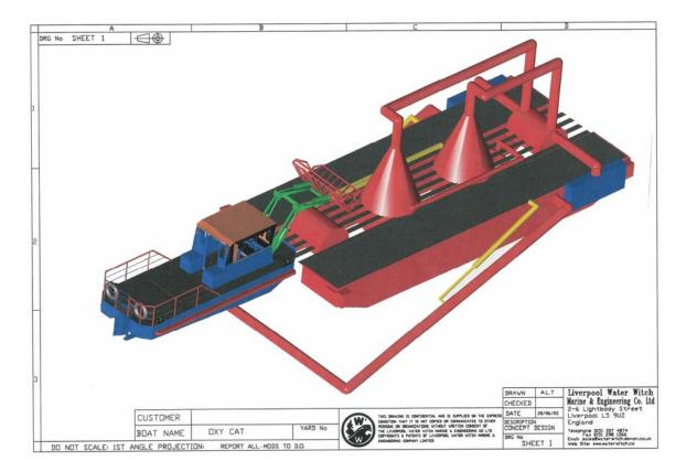
Placement of oxygen within the water column by a variable depth discharge diffuser system.
