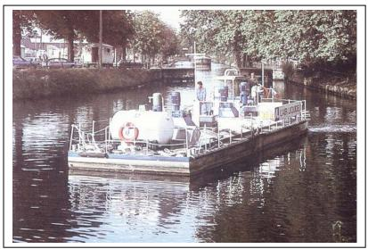
and then discharge it back into the canal. The barge system has been successful in increasing D.O. concentrations in the canals sufficiently to prevent hydrogen sulfide production.
