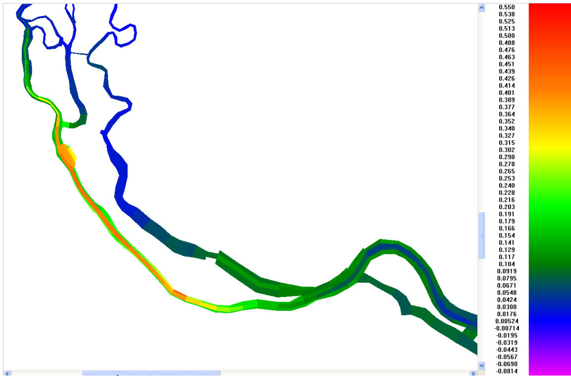
Figure A.1-3 50 th percentile of dissolved oxygen delta distribution in bottom layer of the harbor
