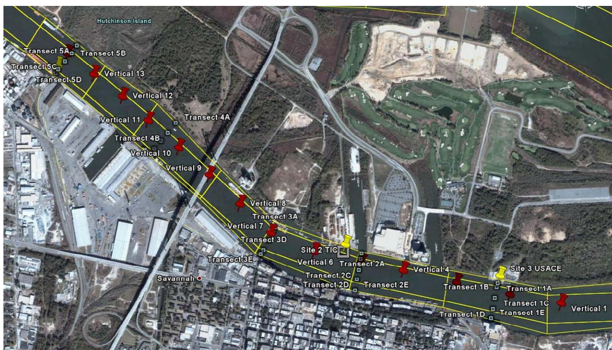
Figure 3-1 EFDC and WASP Model Grid with Summer 2007 Monitoring Stations
