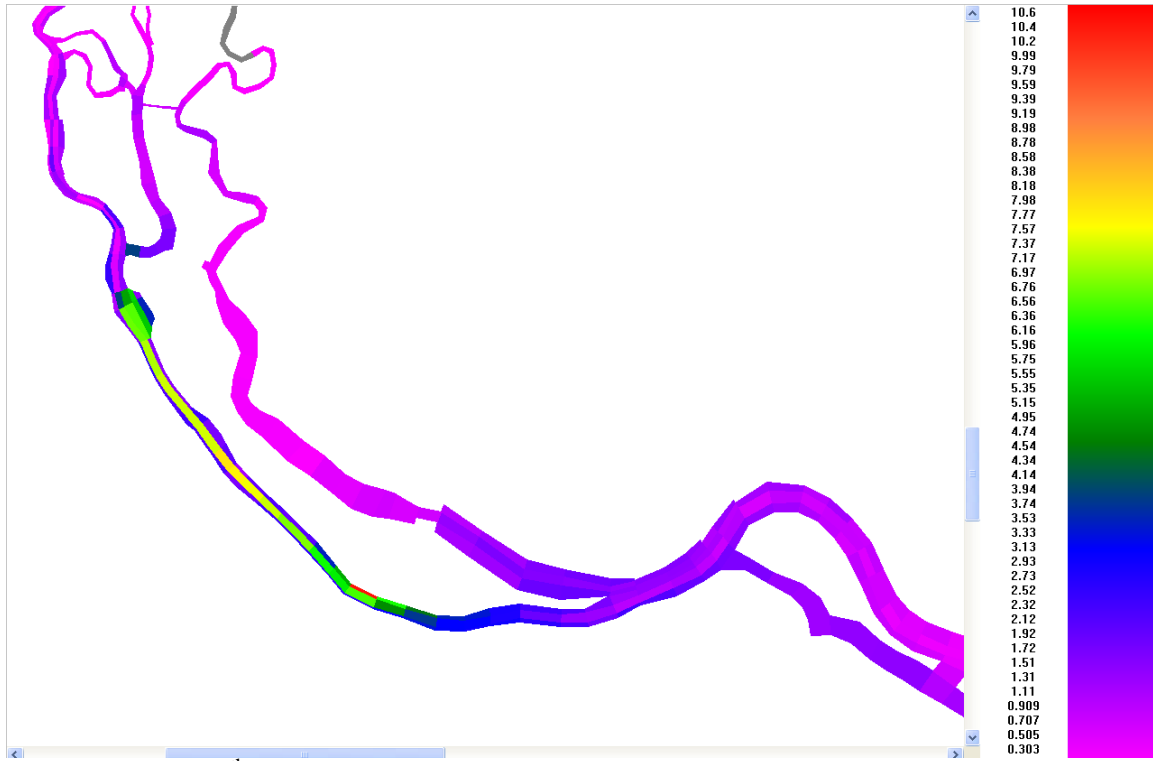
Figure A.3-1 95 th percentile of dissolved oxygen saturation (%) delta distribution in bottom layer of the harbor
