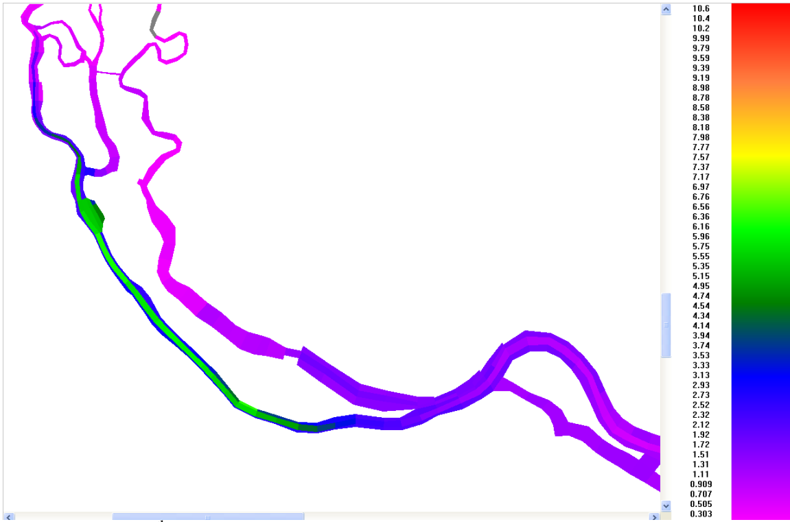
Figure A.3-3 50 th percentile of dissolved oxygen saturation (%) delta distribution in bottom layer of the harbor
