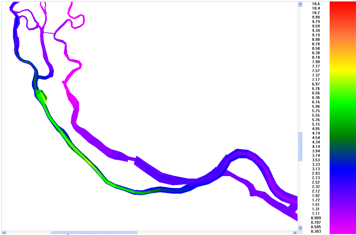
Figure A.3-5 5 th percentile of dissolved oxygen saturation (%) delta distribution in bottom layer of the harbor
