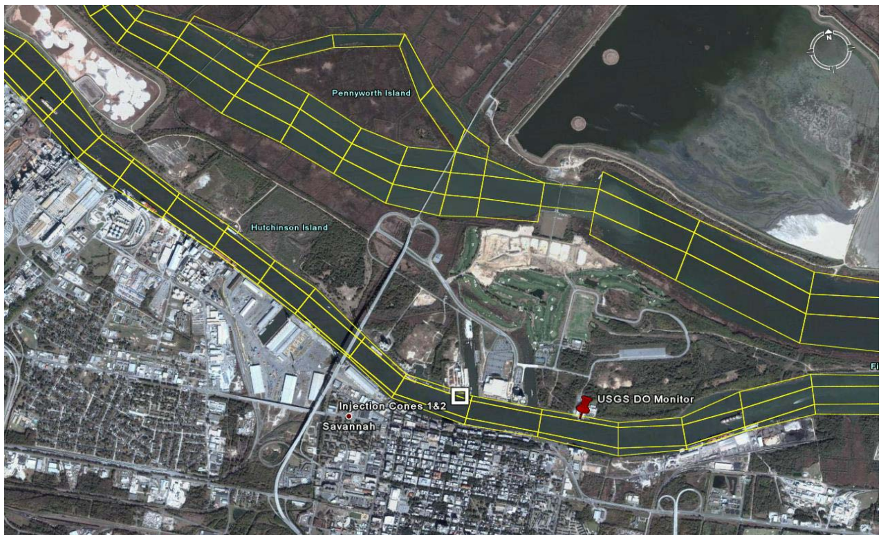
Figure 2-1 EFDC and WASP Model Grid with Injection Point
