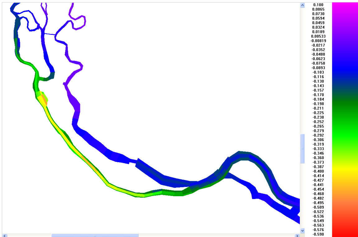
Figure A.2-1 95 th percentile of dissolved oxygen deficit delta distribution in bottom layer of the harbor
