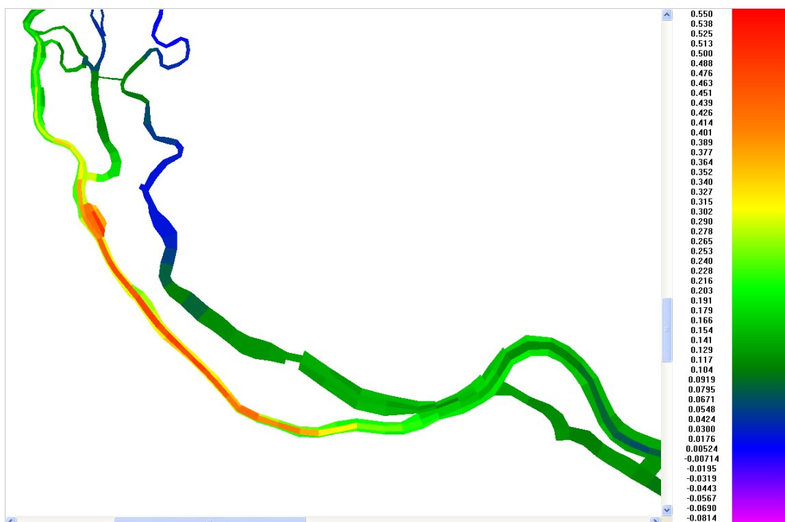
Figure A.1-5 5 th percentile of dissolved oxygen delta distribution in bottom layer of the harbor
