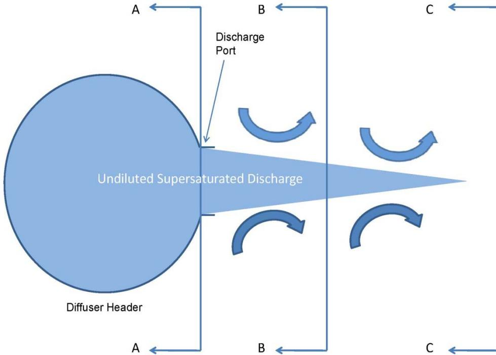
Fig. 4 Schematic of Mixing in Diffuser Jet
