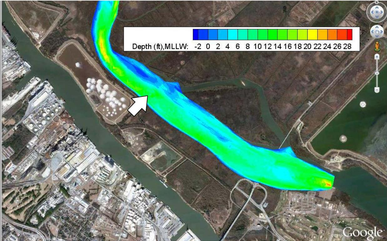
Figure 17 Close-up Bathymetry of Discharge Location (Data collected June 2011, USACE Savannah District)
