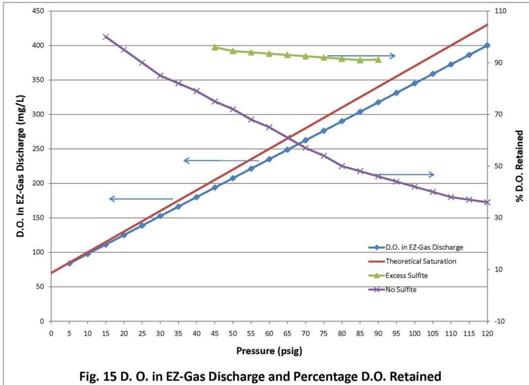
Back pressure studies were conducted in which superoxygenated water was raised to 180 mg/L of D.O. and discharged into a reservoir at the equivalent of 50 feet below the surface and no effervescence loss of D.O. was observed. When water was raised to 140 mg/L of D.O., it could be injected 20 feet below the surface with no effervescent loss of D.O.
