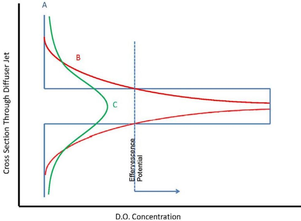
Fig 5. D.O. Profile in Diffuser Jet
