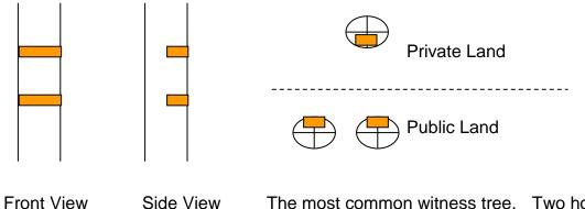
The most common witness tree. Two horizontal hacks face the boundary line. Only trees within 30 inches of the boundary line are marked.
