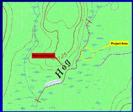
The flow characteristics of a particular tributary will be evaluated at the farthest downstream limit of such tributary (i.e., the point the tributary enters a higher order stream).
