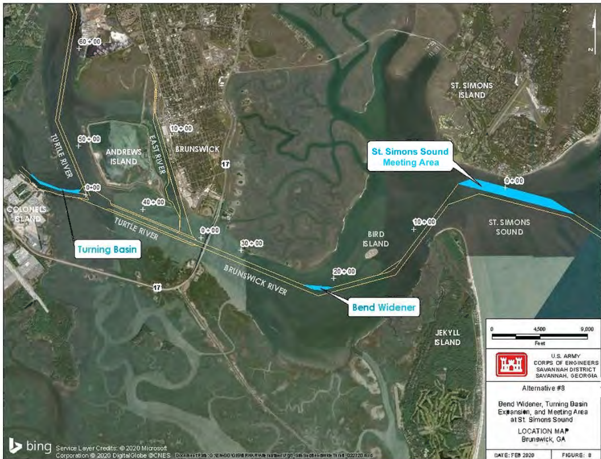
Figure 25. Alternative 8 – Bend widener, turning basin expansion, and meeting area at St. Simons Sound
