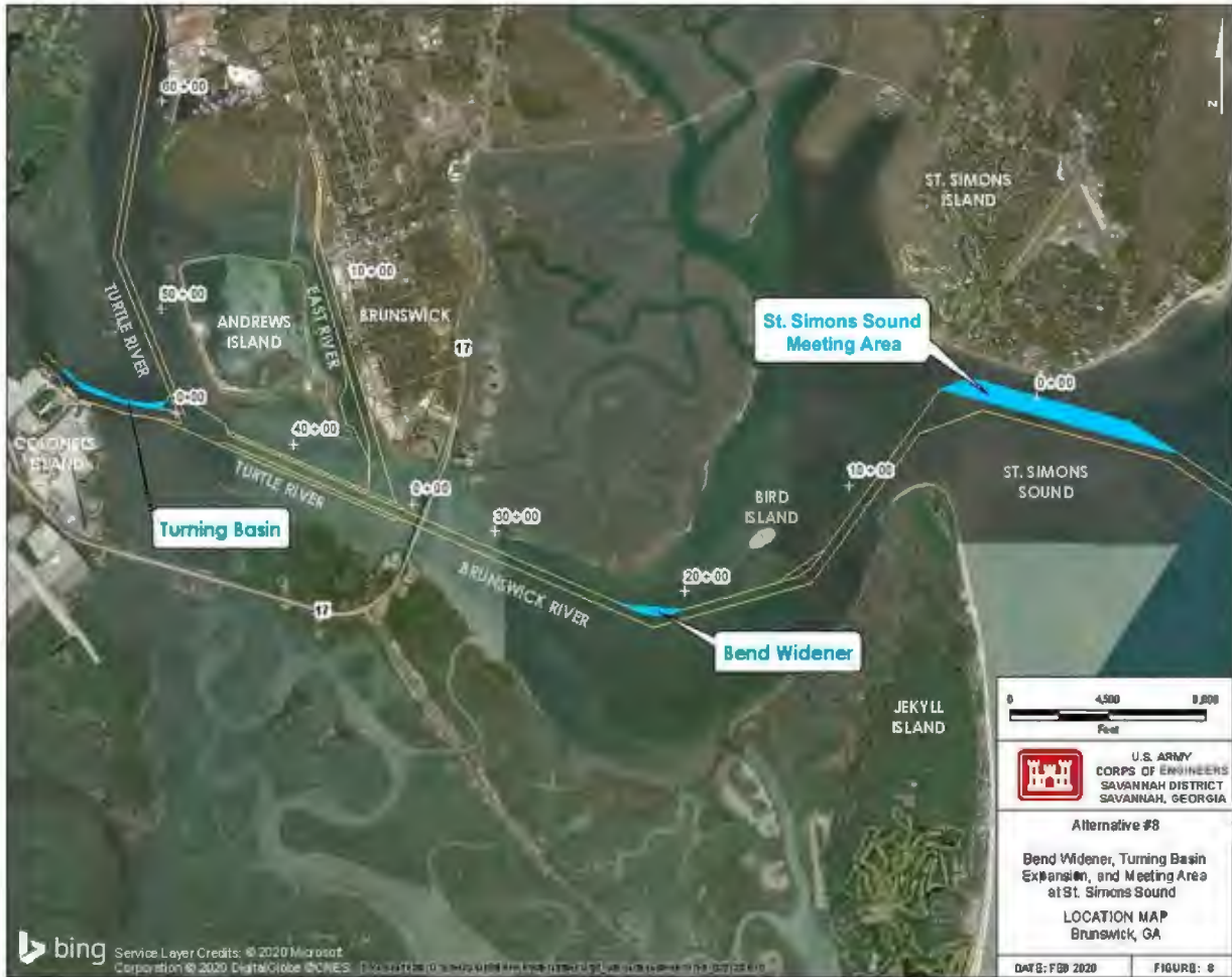
Figure ES.1. Alt. 8 - Bend widener, turning basin expansion, and meeting area at St. Simons Sound. Existing Federal navigation channel denoted by yellow lines with areas of proposed channel widening highlighted in blue.
